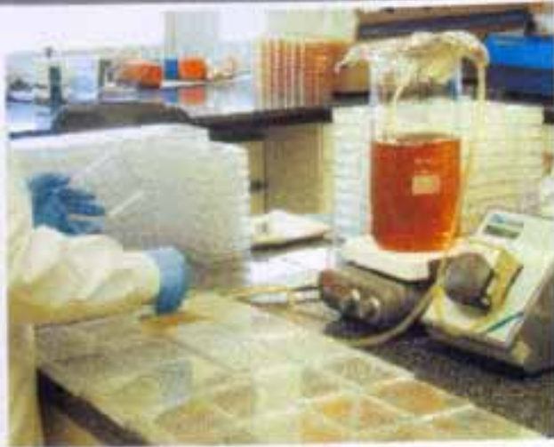
Manual plate filling with peristaltic pump and manifold
