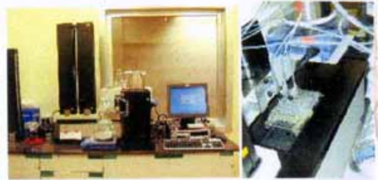
MAP-C2 Agat Dispensing System for filling Corning well, 48-well plates, and 96 well plates (Titertek, Huntsville, AL, USA)
