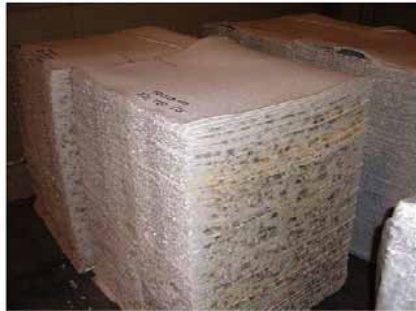
Fig. 5 – Wet Lap contaminated with mold.
