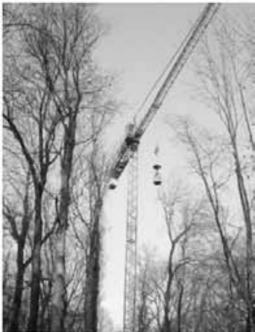
Fig. 1. The construction crane used in the Leipzig Geopark Project (LGP). The small platform is used to access to different levels of the canopy.
