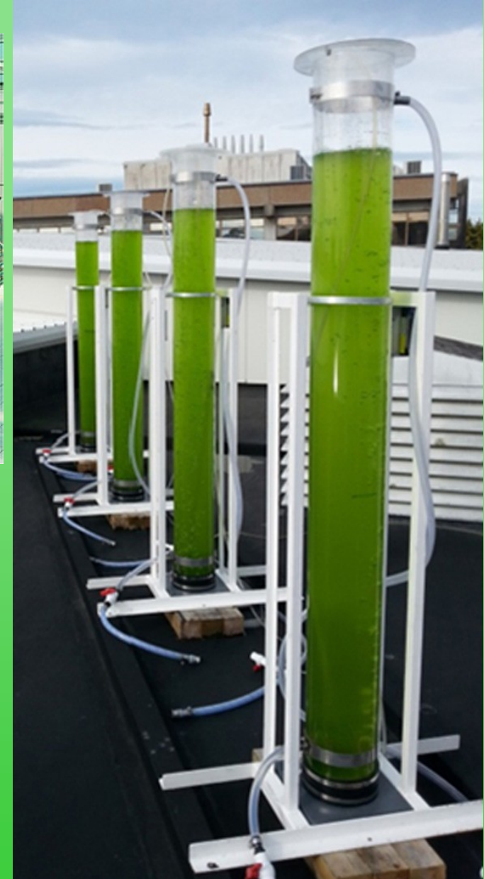
Plexiglas bubble column reactor with diameter 0.2 m, height 2 m, working volume 50 - 60 L
