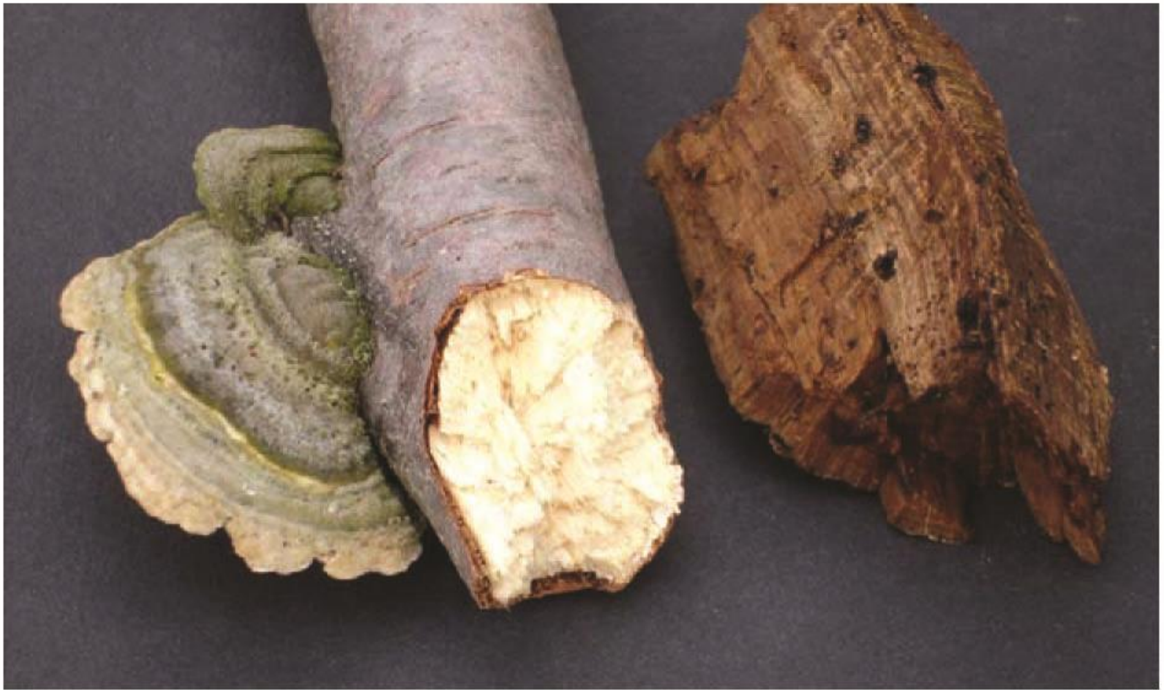
Fig. 2 – Beech wood colonised by the white-rot fungus Trametes hirsuta (left) and by an unidentified brown-rot fungus (right).
