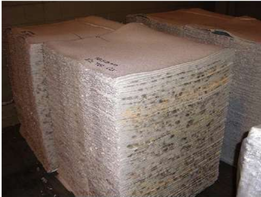
Fig. 5 – Wet Lap contaminated with mold.
