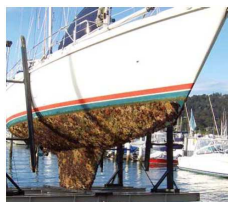
An example of biofouling of algae and invertebrates on a vessel (www.daff.gov.au)
